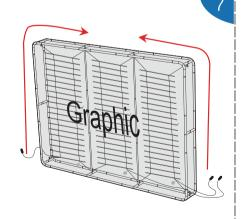
Zip the zipper. Fix the whole frame into the base and lock the slider with allen key
