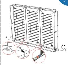
Hang the LED light into the frame sequentially, beware the direction of the LED panel
