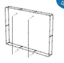
Install the middle tube to finish the frame
