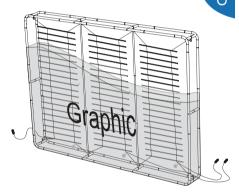
Set up graphic to the frame.( Light power line should be out from holes in graphic; If it's single side printing, the LED direction should face the back of the graphic to achieve better effect)
